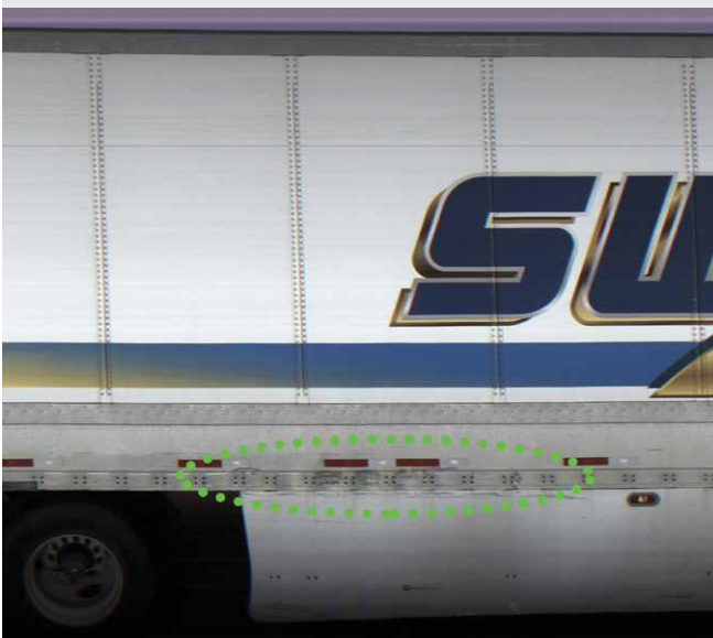
Trailer with damaged bottom rail, often due to lifting operations.
